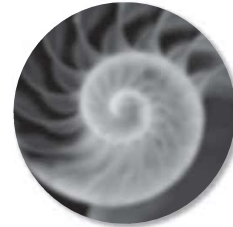
The generator focal spot Y: 0.7 mm
